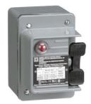
Switch, manual, 30A, 3 pole, 10 HP at 575 VAC, three phase, toggle operated, red 440/600 VAC indicator, NEMA 4 enclosure
